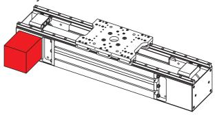
[B] Gearbox on right is fully assembled
