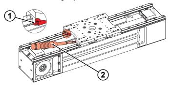
1 Lubrication nipple M6 (DIN 71412 A)
