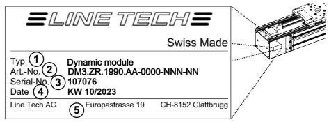
The following information is included on the type plate and makes it easy to identify the dynamic module:
