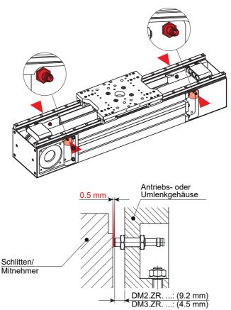
LINE TECH offers inductive limit switches with M8 connectors as standard:
